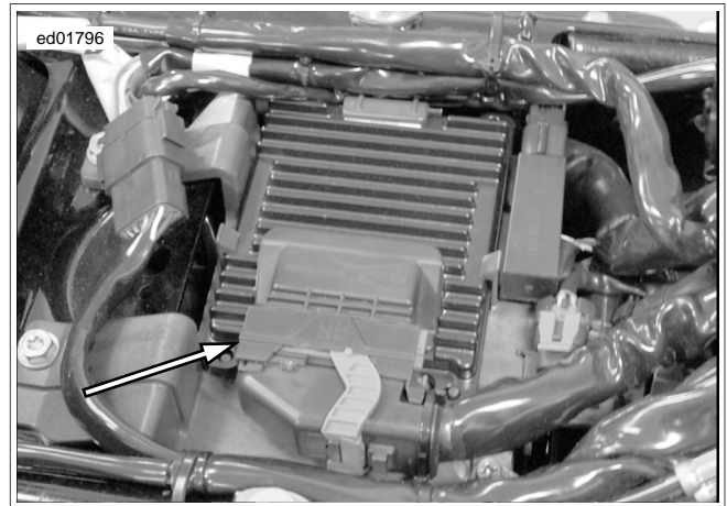
Figure 4-67. Electronic Control Module (ECM)
