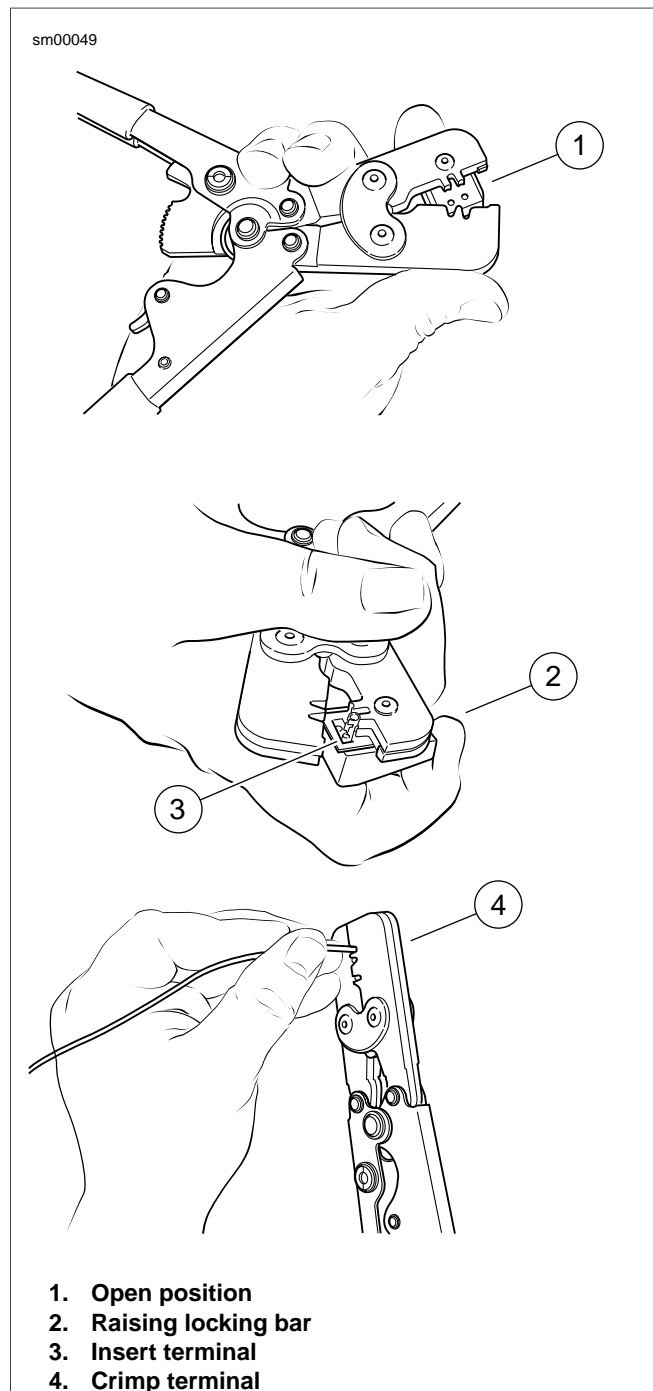
Figure A-46. Packard Micro 64 Connector: Terminal in Crimper
