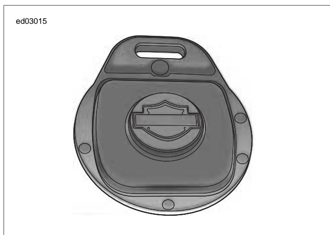
Figure E-29. Key Fob Assembly: TSSM
