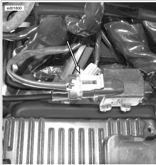
Figure B-14. [95] Purge Solenoid (Under seat)
