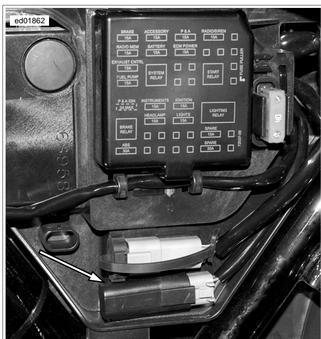
Figure 6-4. ABS Diode Pack
