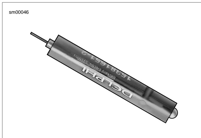
Figure A-42. Packard Micro 64 Terminal Remover (HD-45928)
